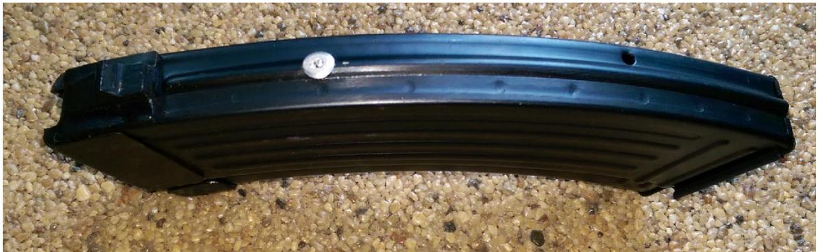
*Re: Point 4. An AK 30 round magazine that has been blocked at 5 rounds in order to conform to Italian regulations by means of a simple rivet. This can easily be re-converted with a simple drill so that the magazine will hold 30 rounds again.*
